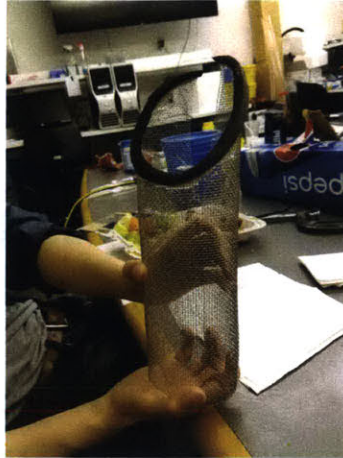
Figure 2-17: Wire mesh for robot retrieval
