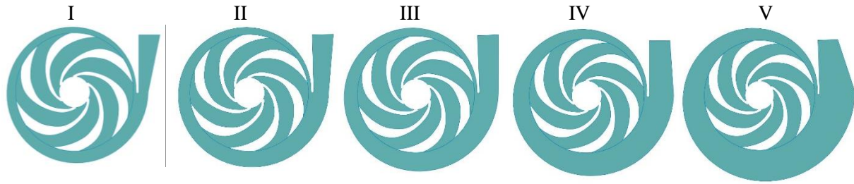
Figure 8. Five different volutes used for analysis. The only dimension changed between the volutes is the throat area, and the resulting volute height around the spiral. Changing the throat area, in essence, changes the size of the “wedge” inserted into the volute in Figure 5. It changes the volute cross-section and impacts the flow.
