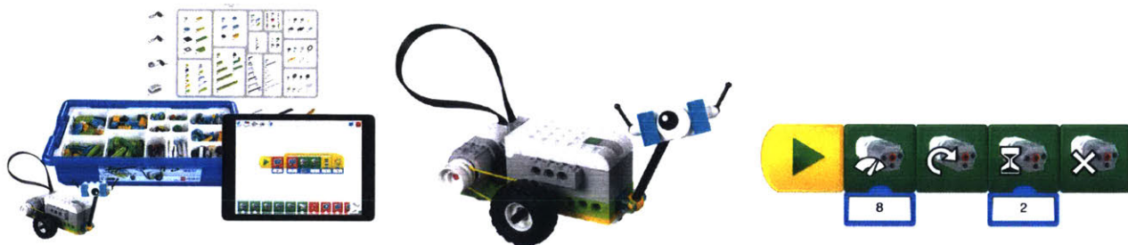
Figure 16.a. WeDo 2.0 construction kit. 16.b. Rover using a sensor and a motor constructed using WeDo 2.0 blocks. 16.c. Visual programming interface used to program the WeDo controller.
