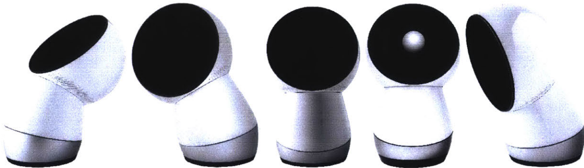
Figure 4. Different poses of the Jibo robot that enables the generation of animations and emotional expressions.
