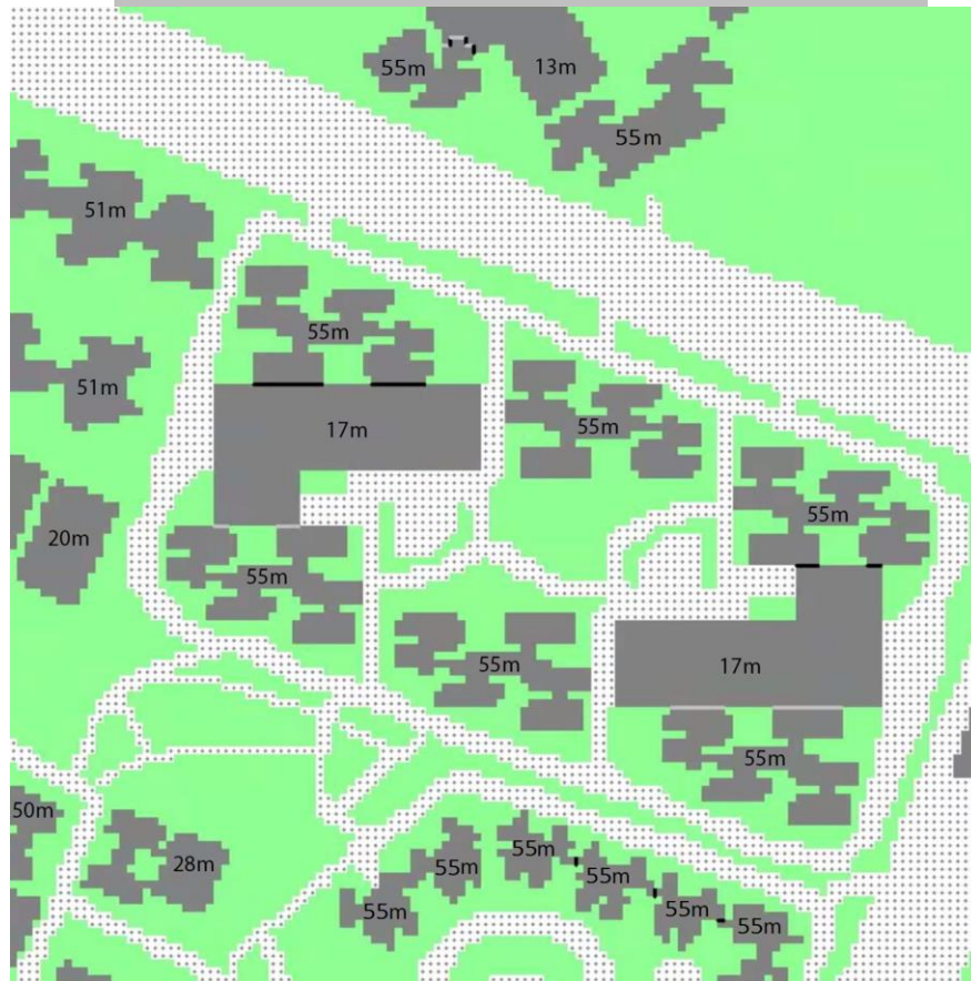
Fig. 2 Modelled spatial domain including building footprint and height, and vegetation (grass)
