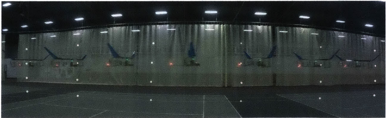
Figure 6-4: Time lapse of EAD aircraft in-flight. White reference markers are spaced 5m horizontally and 1m vertically. All results in Fig. 6-5 are presented in a Cartesian coordinate system with the x axis in flight direction, z axis upwards, and y axis pointing away from the camera (illustration by Haofeng Xu).
