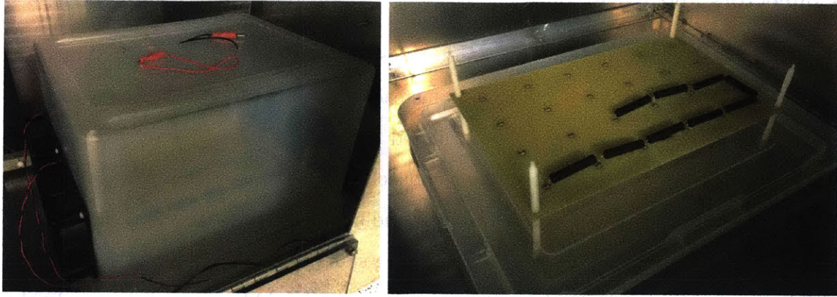
(a) Resistor load box enclosed. The leads of (b) Resistor load printed-circuit board. One can easily swap different resistors in. PCBs can be stacked vertically on top of each other through four standoffs. The box to blow air on the resistors.
