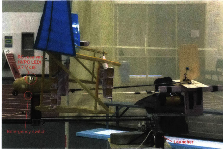
Figure H-2: The assembled EAD aircraft sitting on the launcher. The HVPC LED indicator turns green when high voltage (HV) off, blue when charging the input caps and red when HV on. The emergency switch mounted at the bottom of the fuselage is in-line with the logic power to the HVPC. Landing triggers it and cuts off the logic power.
