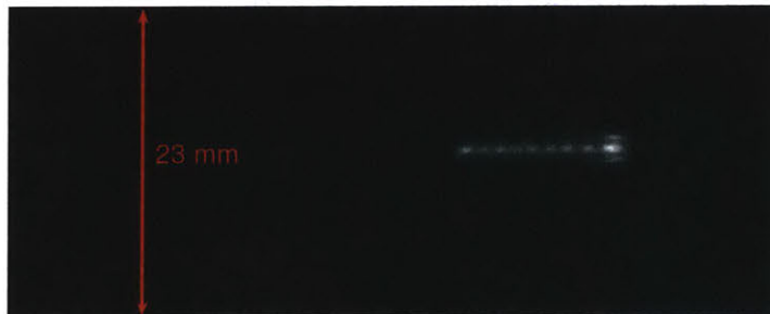
(c) Visible light emission from multipactor on an alumina rod
