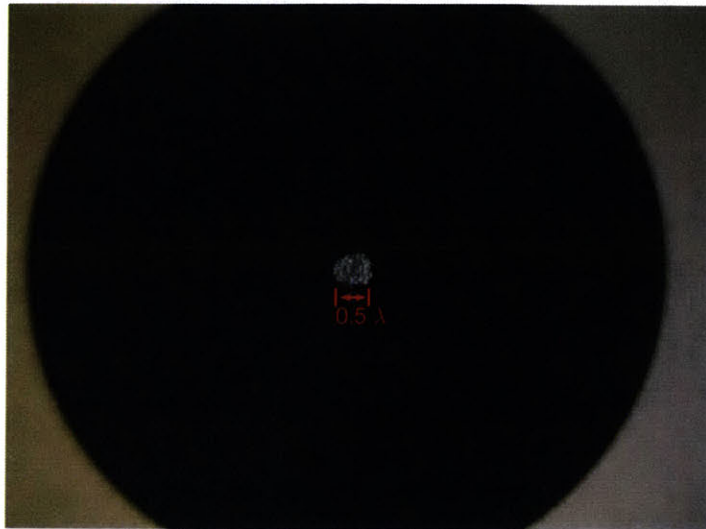
Figure 6-14: Observed damage to high resistivity silicon tested with tangential electric fields. In testing, the material was steadily eroded by breakdowns until the Fabry-Perot cavity was out of resonance. However, no energetic electrons were collected by the dark current monitor, indicating that the failure was not due to the formation of multipactor. Damage was observed on only one side of the wafer, where the electric field was highest. Two samples were tested with the same result.
