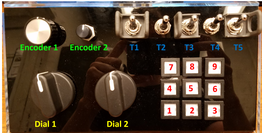
Figure 2-6: Switchboard tactility task with control types annotated
