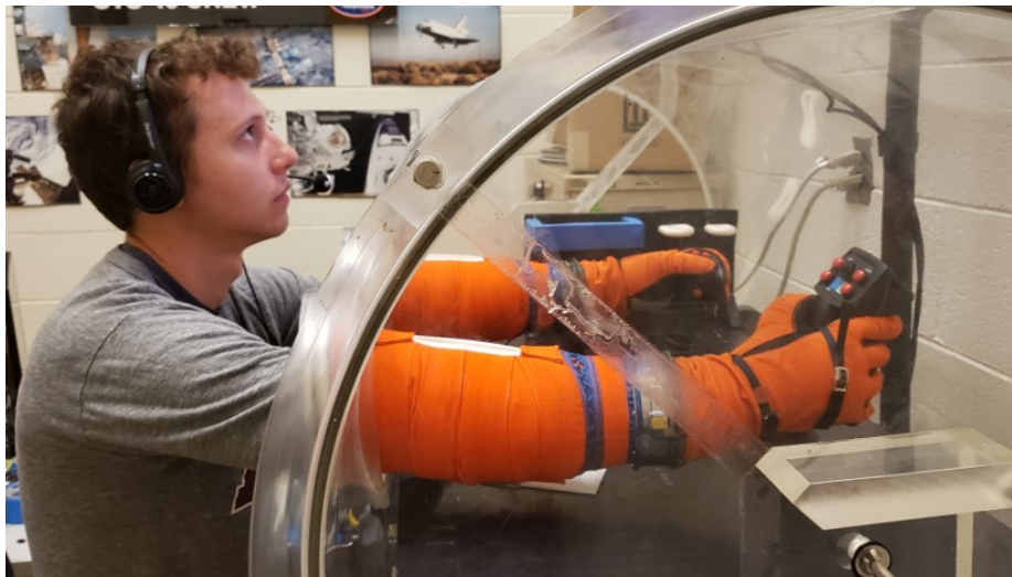
Figure 2-3: Subject performing lunar landing simulator task in glovebox vacuum chamber
