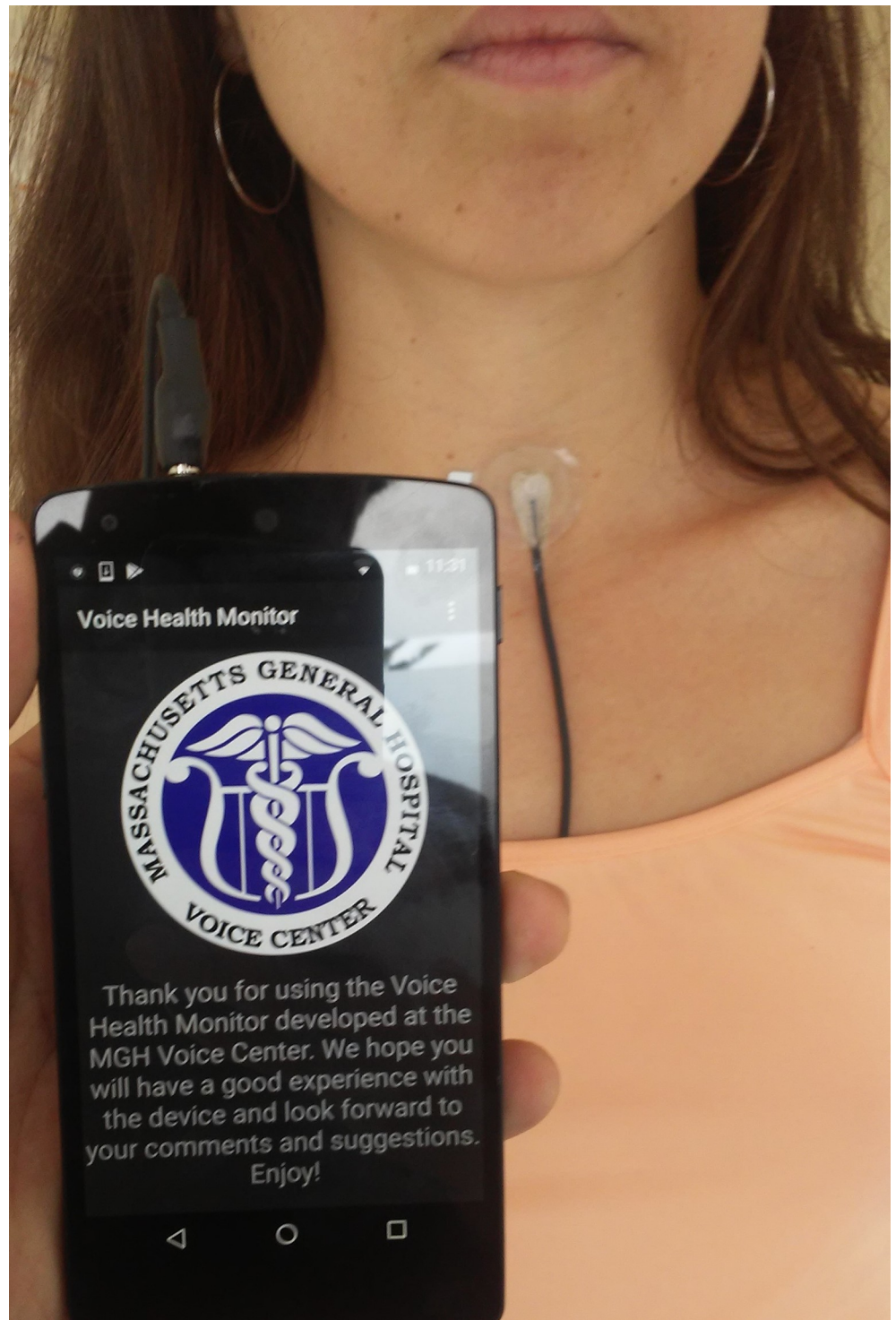
Fig 1. Example of VHM system. Illustration of the smartphone-based ambulatory voice monitor that uses a neck-surface accelerometer attached to the skin halfway between the thyroid prominence and the suprasternal notch of a female subject.
