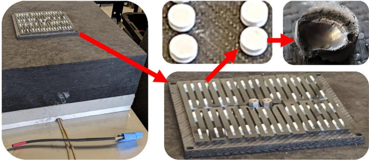
Figure 3.3: Hafnium oxide electrical insulators reduced by carbon. The white discs made from hafnia ( \text{HfO}_2 ) were reduced to hafnium when heated to 2000°C in the presence of solid carbon beneath them, and gaseous evaporated carbon surrounding them.
