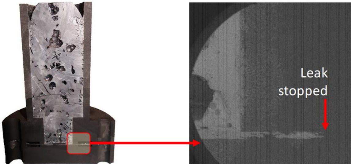
Figure 4.8: Self-sealing behavior of SiC reaction. After leaking 1 mm along the seal path, the leak was blocked by the formation of SiC.
