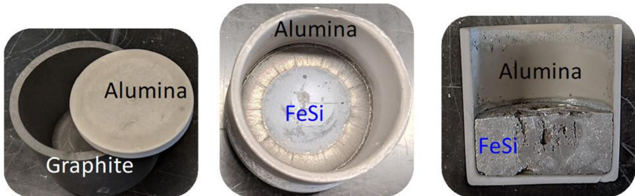
Figure 4.16: FeSi ingots pre-melted in alumina, heated inside graphite for induction heating
