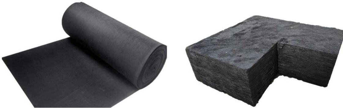
Figure 2.4: Graphite insulation. On the left a flexible graphite felt is shown while on the right a rigid graphite board is shown. The rigid material is most expensive and slightly more conductive, so it is often used only where compressive strength is needed.
