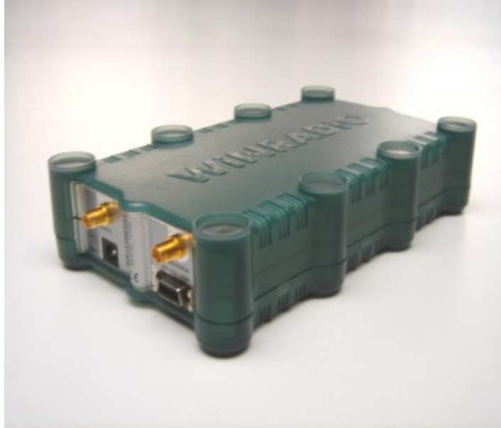
Figure 3-5: A WiNRADIO G39WSBE software-defined receiver (image from www.winradio.com/home/g39wsbe.htm ). Ports on the front-left face of the receiver are: (top left) analog audio out (SMA), (top right) VHF in (SMA), (bottom left) power (2.5 mm), and (bottom right) digital audio out (serial).
