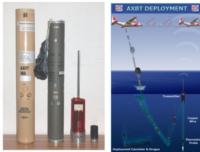
Figure 2-1: (Left) components of an AXBT (from left to right: storage canister, AXBT casing, surface float, and thermistor probe) and (right) a typical AXBT deployment diagram. Figure from www.hurricanescience.org/science/observation/aircrafttrecon/expendableairborneinstruments/ (images originally provided by the USCG International Ice Patrol).
