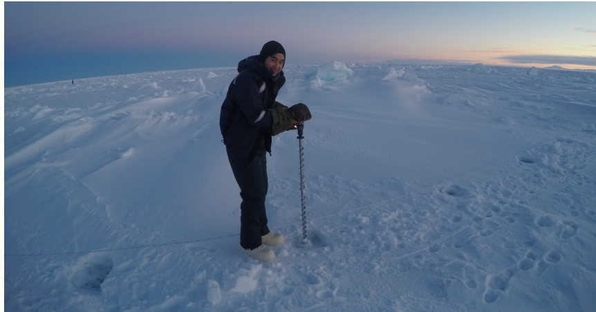
Figure 2-4: An example of a drill line during PIPERS. At each drill location (spaced 2 m apart), a small area is cleared of snow for ease of drilling, clearly visible here. Drill sites tend to be selected for their ease of access, and so are biased towards thinner and flatter ice.
