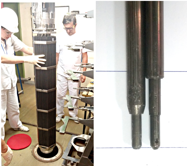
Figure D-3: Left: a fuel assembly for the LR-0 reactor at CVŘež. For scale, note the workers handling the assembly. Right: the lower end of two different fuel pin designs for the LR-0 assemblies. The upper of the two lines in the background indicates the bottom of the \text{UO}_2 fuel in the interior.
