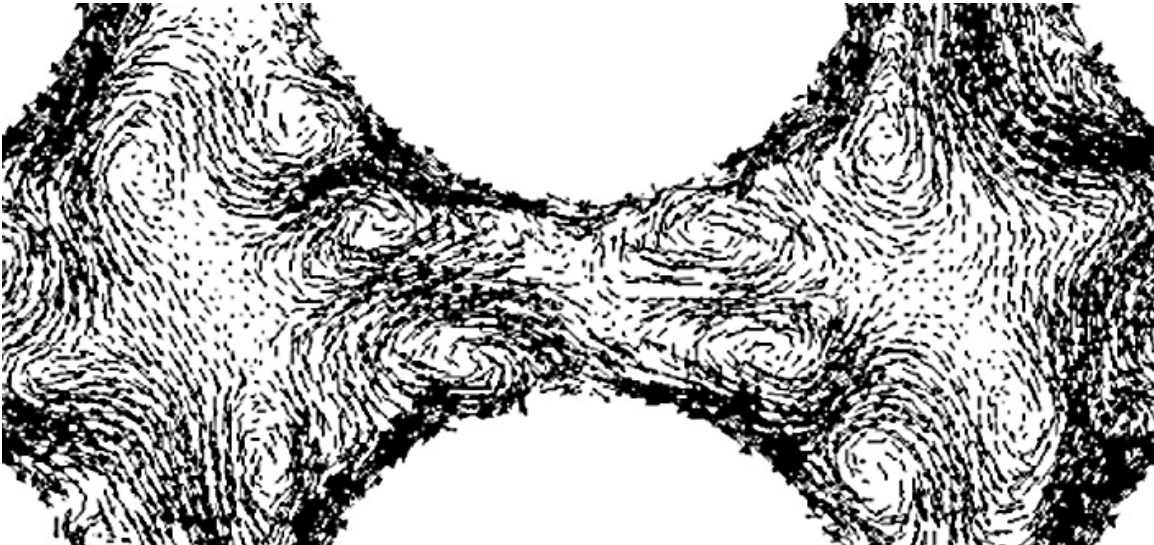
Figure 2-7: Plot of instantaneous velocity from an LES simulation of a bare rod bundle. Vortices can be seen near the gap that are representative of the mean secondary flows. Image from [14].
