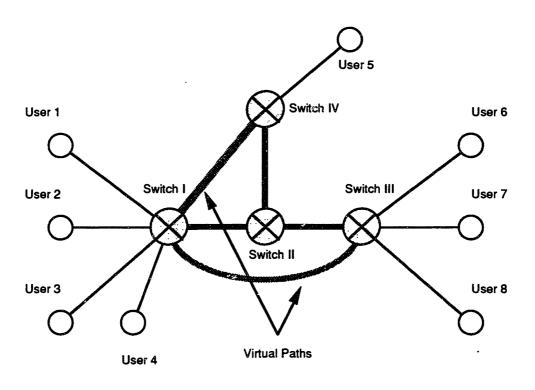
The dark lines represent physical paths connecting the ATM switches.
