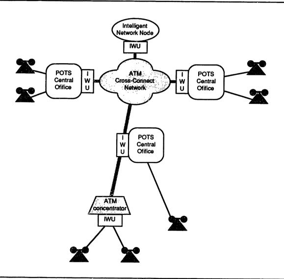
ATM virtual paths are used to connect the central offices and an ATM concentrator is used to transport some subscriber traffic to a central office.
