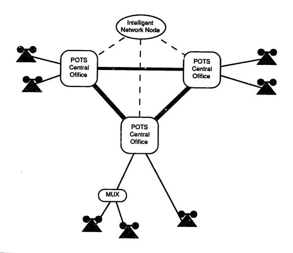
Figure 5.2 shows an early phase of the introduction of ATM into the network. The most notable difference from the contemporary network is the replacement of the direct trunks
