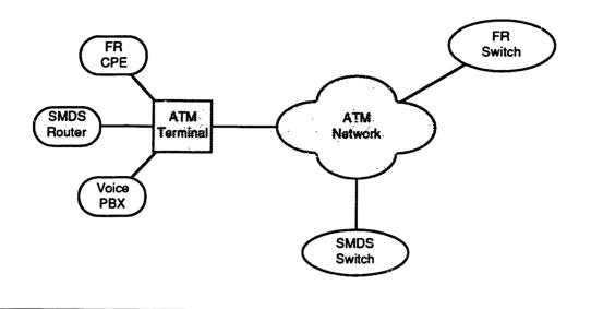
Figure 7.3. Frame Relay providing access to an ATM network.
