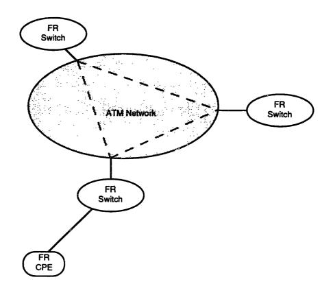
Figure 7.2. ATM as an integrated on-ramp, providing access to different communication services.
