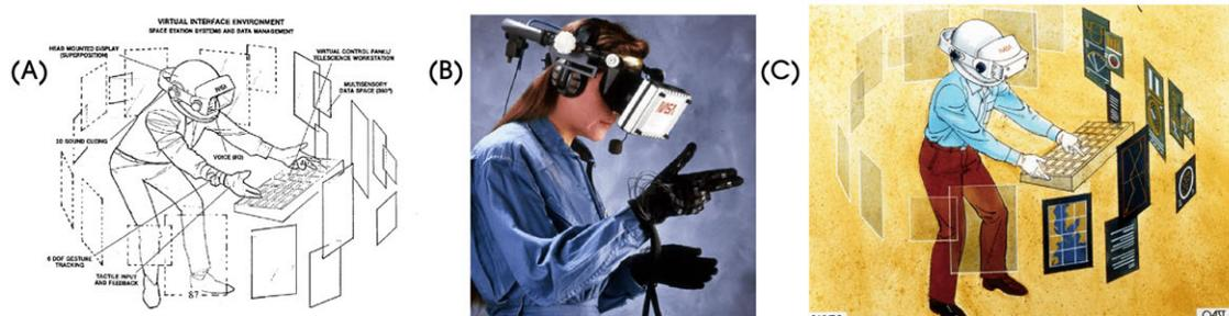
Figure 11: VIEW Project shown. (a) shows a schematic of different components of VIEW, including virtual control panel, 360 degree data space, 6DoF gesture tracking, tactile input, voice interface, and 3D sound cues. (B) shows a user wearing the VIEW hardware. (C) shows a colored rendering of the manipulable data panels. Image Credit: NASA/W.Sisler, S. Fisher, 1988
