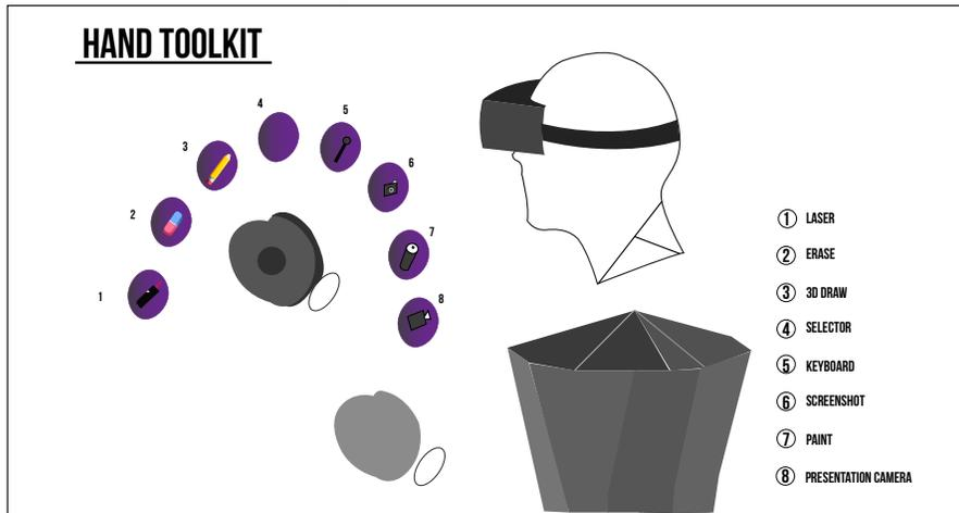
Figure 30: Hand toolkit being used. On the user's right hand are 7 buttons arranged in a semi-circle. This is the hand-toolkit an avatar-space interface.
