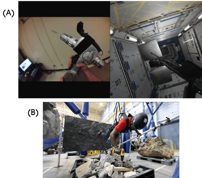
Figure 13: Hybrid Reality lab at Johnson Space Center. (A) shows a physical drill prop on the left and a virtual model mapped one-to-one in VR. (B) shows the ARGOS system as a trainee performs a drilling task while suspended in simulated micro-gravity.
