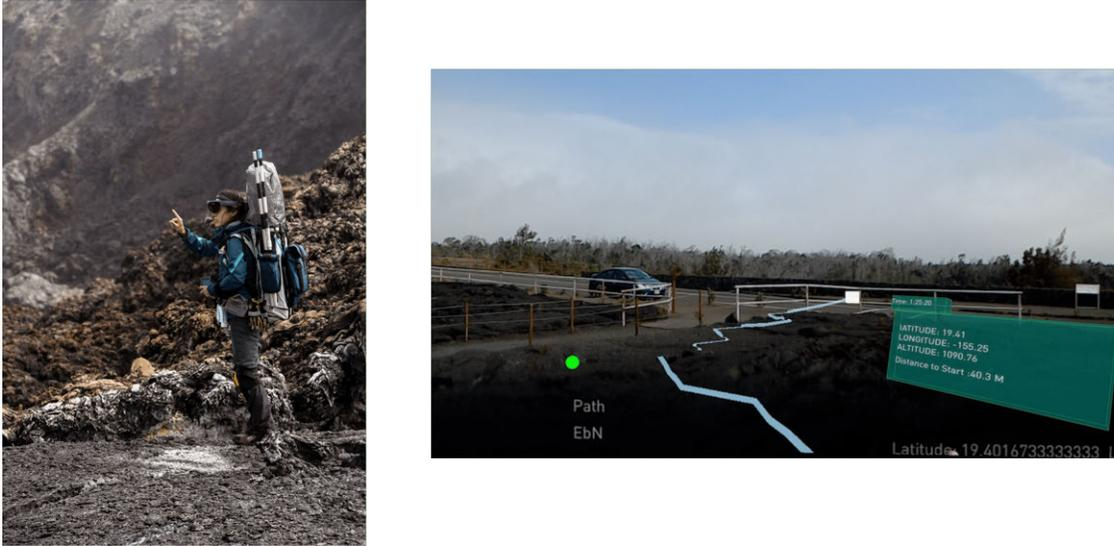
Figure 7: Holo-SEXTANT in use during the BASALT-3 field deployment. (a) shows crew member calibrating their path and traverse. (b) shows a through-the-headset view of the augmented reality path and navigational information
