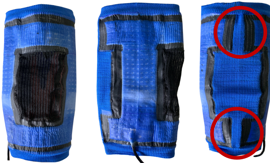
Figure 3-11: Anterior (left), lateral (center), and posterior (right) views of soft knee exoskeleton V1 with insufficient elasticity of base fabric separating posterior airbags (circled).
