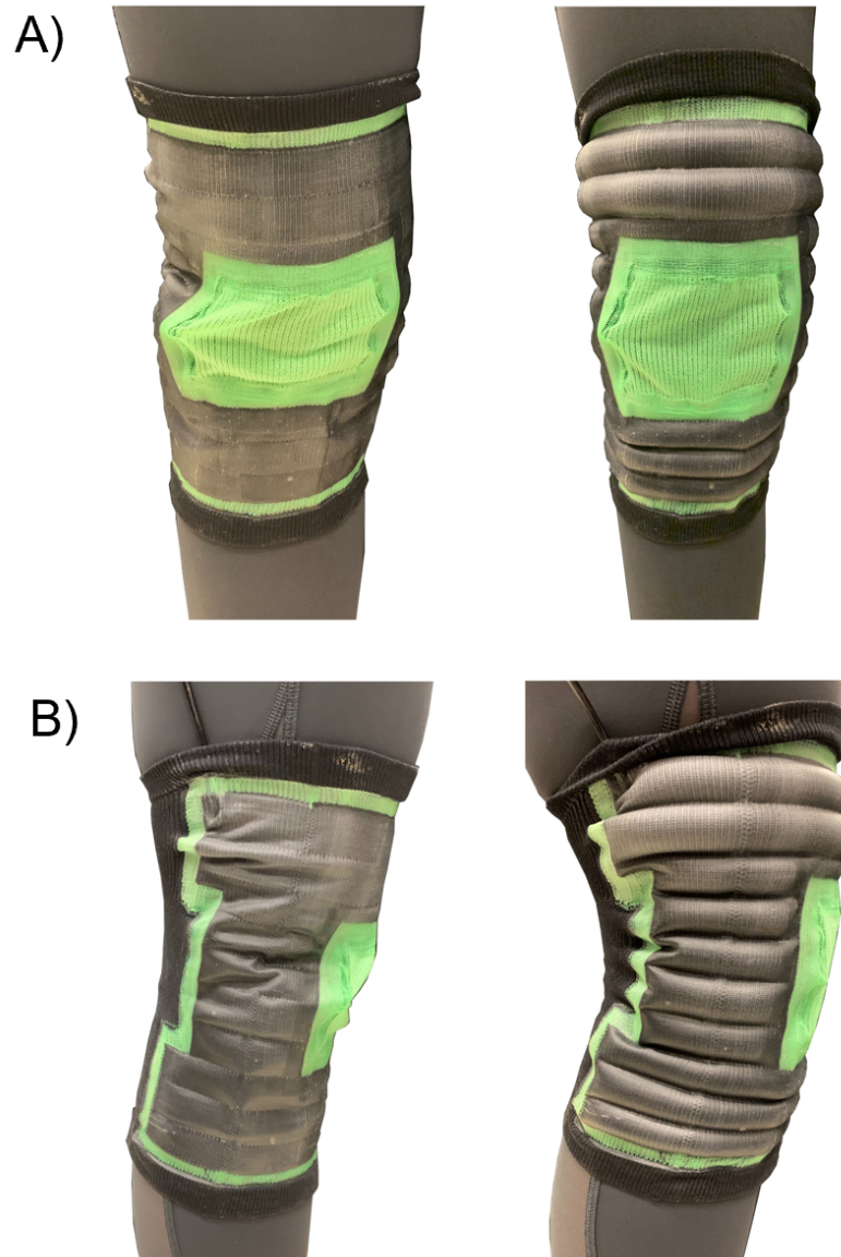
Figure 3-13: Soft knee exoskeleton V2 donned (left) and maximally inflated (right). A) Anterior view. B) Lateral view.
