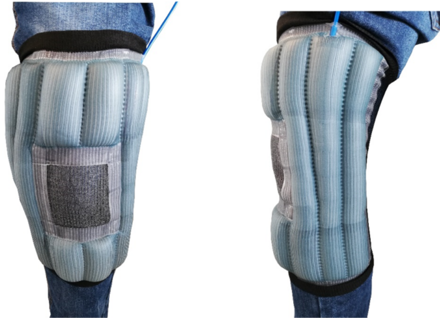
Figure 3-14: Soft knee exoskeleton V3 donned and maximally inflated anterior (left) and lateral (right) views.
