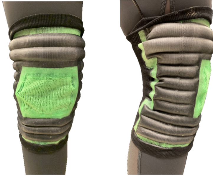
Figure 4-1: Soft knee exoskeleton V2 donned and maximally inflated anterior (left) and lateral (right) views.
