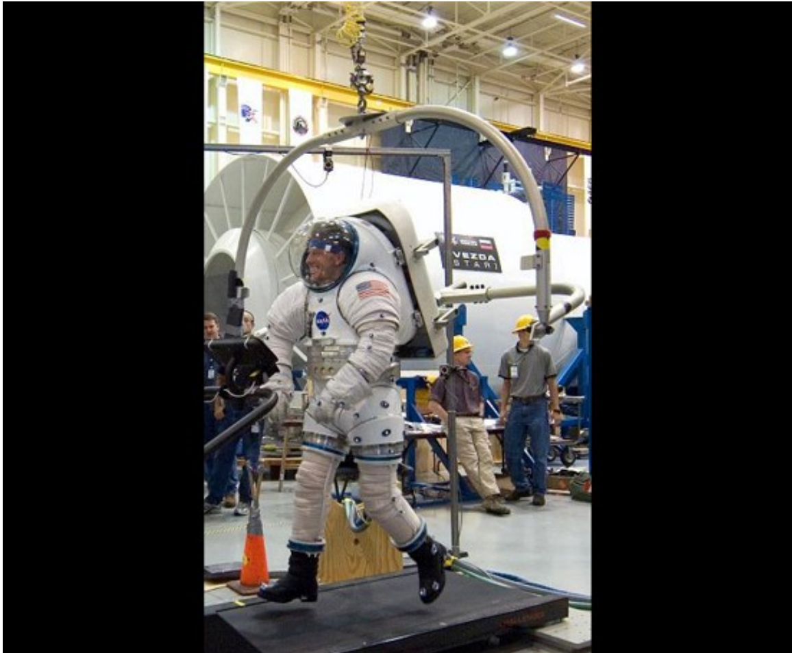
Figure 3-23: A subject performing a treadmill locomotion task using the POGO partial gravity simulator during an EVA study (NASA, 2020).
