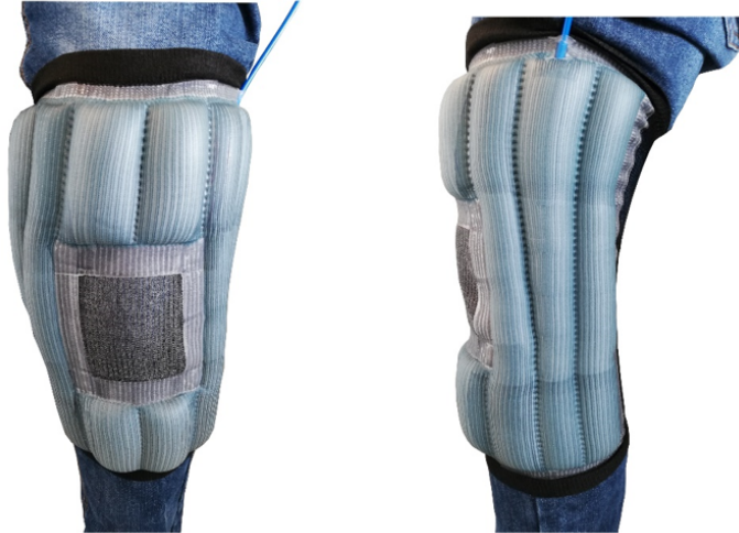
Figure 4-2: Soft knee exoskeleton V3 donned and maximally inflated anterior (left) and lateral (right) views.
