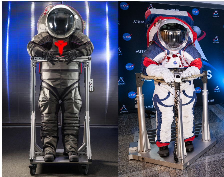
Figure 2-5: A) NASA Z-2 prototype. Image credit: (McFarland, 2016). B) NASA xEMU ground prototype. Image credit: NASA.
