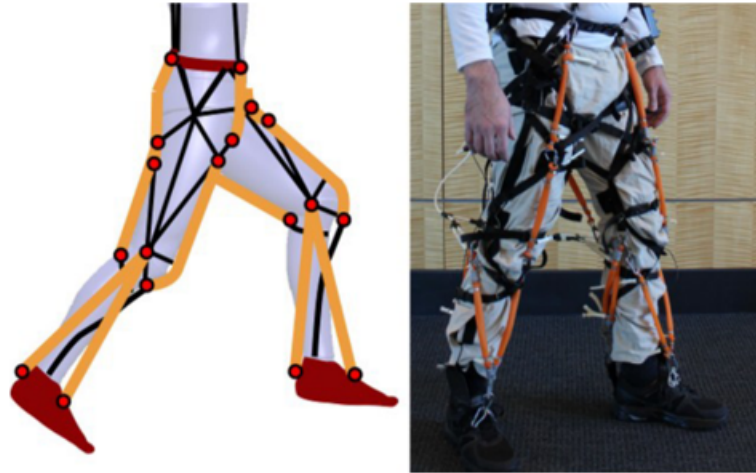
Figure 2-15: Soft exosuit utilizing pneumatic actuators. Image credit: (Wehner et al., 2013).
