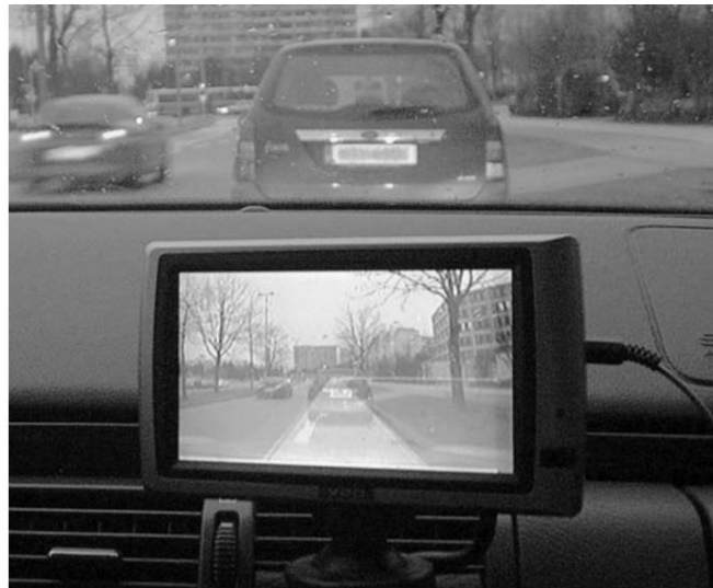
Figure 2.7: 'Video See-Through' AR display used for navigation (Narzt et al., 2005)
