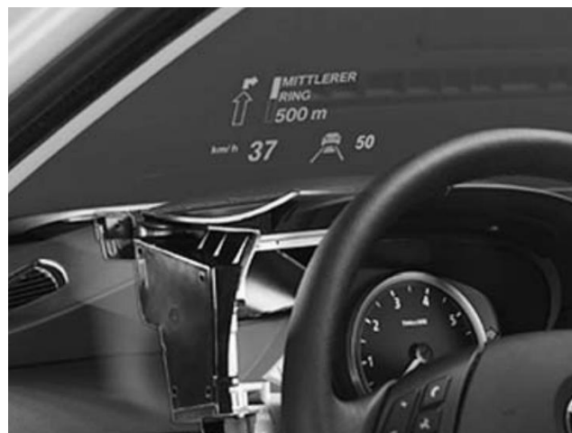
Figure 2.6: ‘Optical See-Through’ AR display on the windshield of a car (Narzt et al., 2005)
