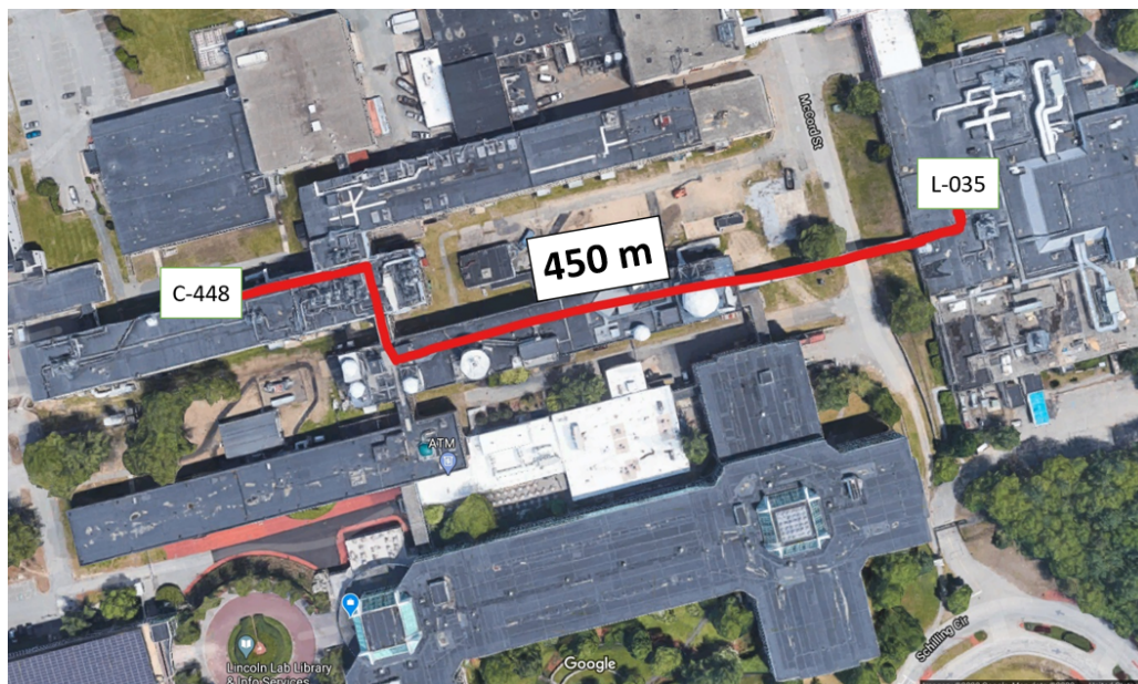
Figure 5-4: Aerial view of the deployed fiber between the Group 67 lab C-448 and Group 89 lab L-035A. This map is oriented with North pointing up.
