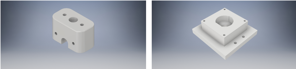
(a) Diagram of stainless steel holder which held the tip in place while connecting it to the pins and the rest of the mount. (b) Diagram of PEEK mount used to attach the rest of the setup to the vacuum chamber.
