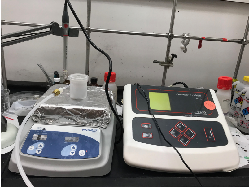
Figure 3-6: Picture of the heating setup. On the left there is the heating plate, the dry box connected to the nitrogen and the conductivity meter probe. On the right, is the conductivity meter.
