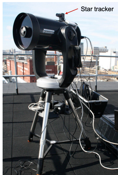
Figure 1-7: Portable optical telescope (PorTeL) used for CLICK mission [24].
