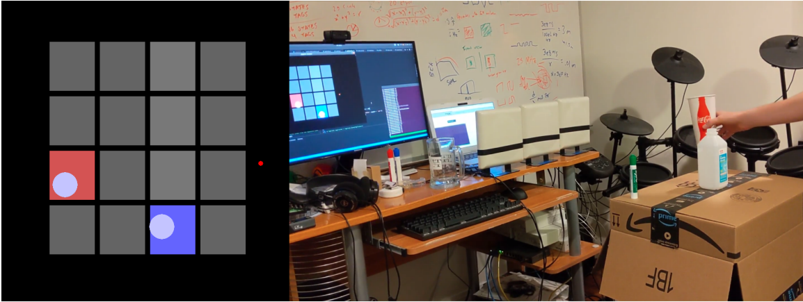
Figure 6-1: The Sequencer/Synthesizer in action. In the application (left), the large white circles represent the objects controlling the sequencer, while the small red dot represents the object controller the synthesizer. These objects, and the surrounding environment, are shown in the photo (right).
