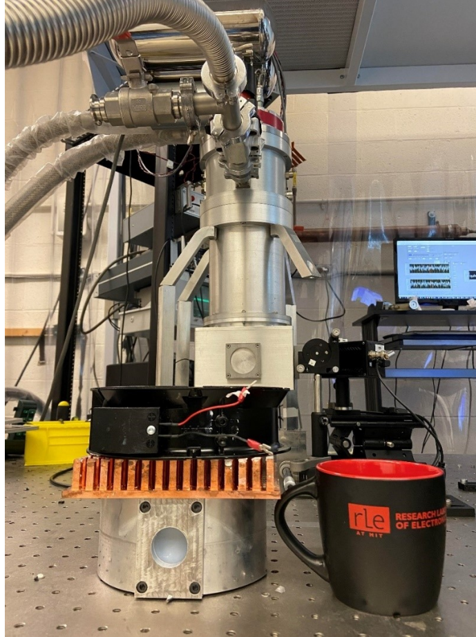
Figure 5-7: Single stage fan-cooled TEC assembly with 4.5” diameter and 6” height. A pulse tube cooler which is commonly used in a laboratory environment is also shown in the background without showing the required pumps and Helium compressor. The hole spacing on the optical table is 1 inch.
