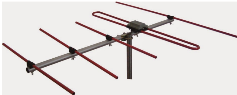
Figure 2-10: a Yagi-Uda (more correctly Uda-Yagi antenna) with three directors and one reflector. The director elements produce destructive interference in minor lobe direction.
