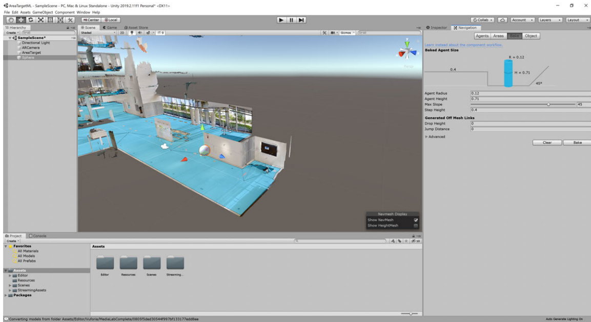
Figure A-16: Bake to obtain navigation mesh of the area target. Play around with the agent settings to generate more appropriate NavMesh surfaces.
