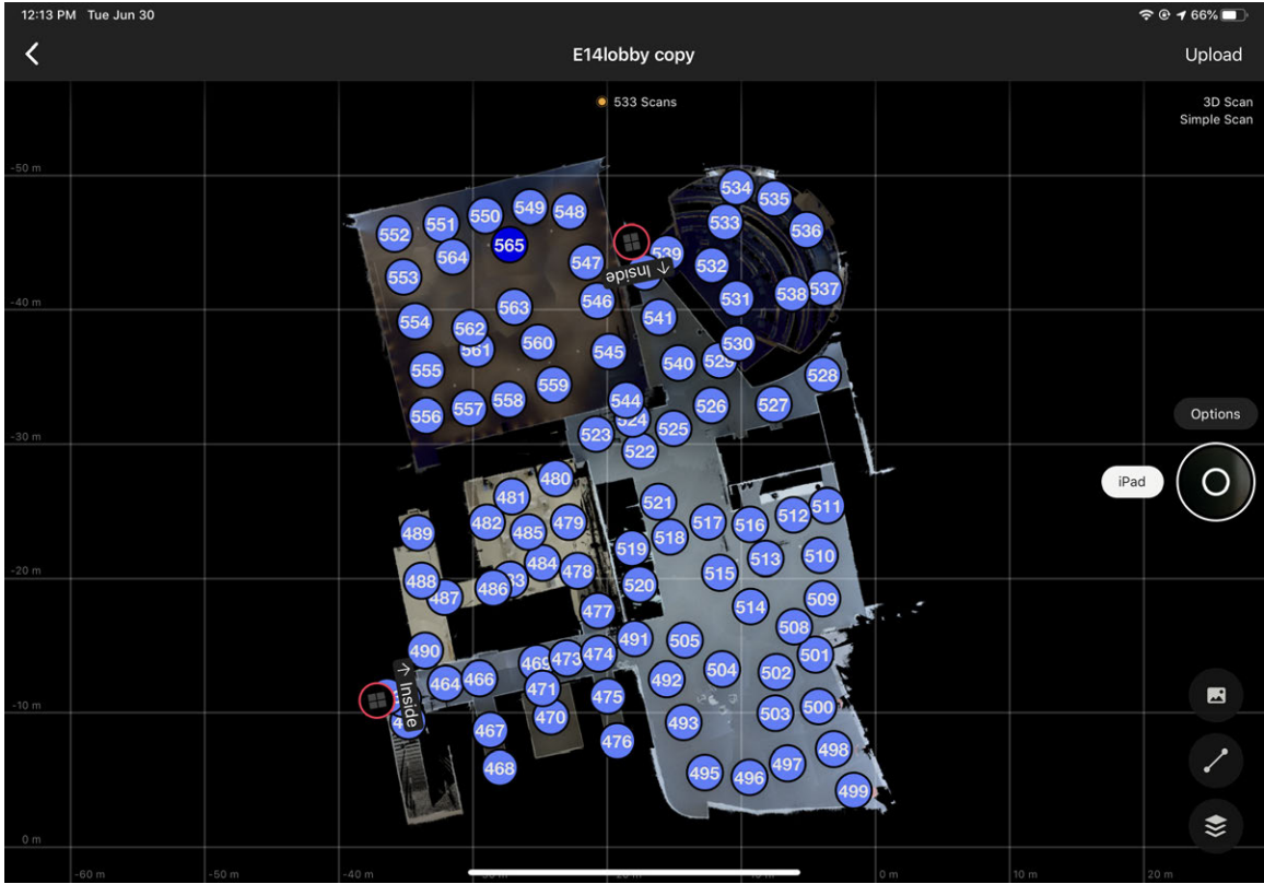
Figure 5-9: 565 scans were made to generate a complete 3D scan of the MIT Media Lab.
