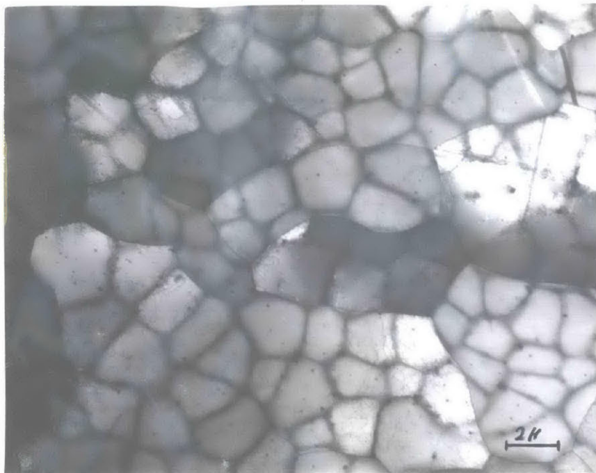
Figure 4.1.--Micrograph of a splat cooled 316 SS containing 100 appm boron taken by a TEM, 5000x.
