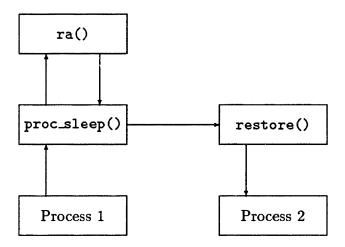
Figure 2.1: A process swap, initiated by a call to proc\_sleep(). Up arrows indicate calls, down arrows returns.
