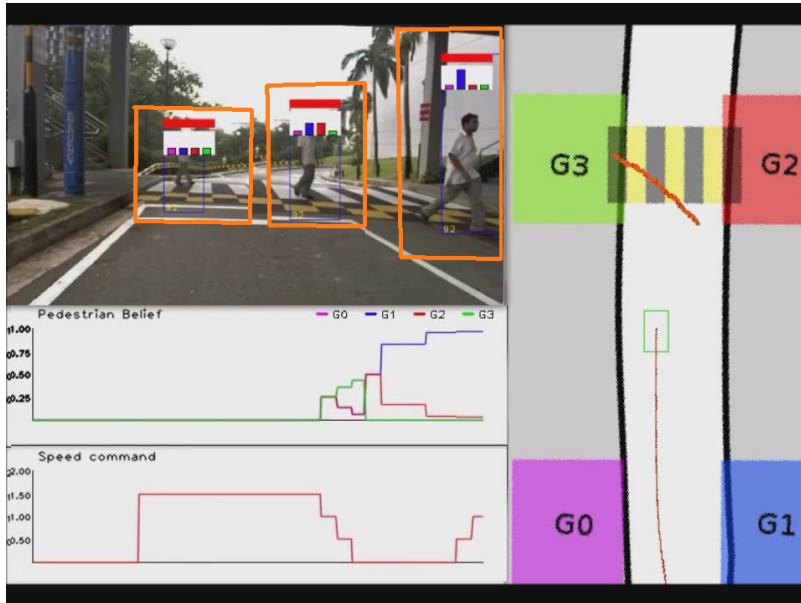
(b) Avoidance for a single pedestrian (on-board camera picture merged at different times to show the evolution of the belief)
