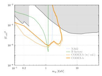
Fig. 35 Projected sensitivity of CODEX-b to Dirac heavy neutral leptons for  $U_{\tau N} \gg U_{eN}$ ,  $U_{\mu N}$  for a tracking detector only (solid) compared to an optimistic case (dashed) with a calorimeter capable of reconstructing the  $N \rightarrow \nu \pi^0$  final state, assuming the background differential flux of single  $\pi^0$ 's is negligible or reducible
