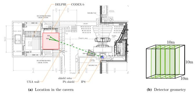
Fig. 3 Left: Layout of the LHCb experimental cavern UX85 at point 8 of the LHC [9], overlaid with the CODEX-b volume, as reproduced from Ref. [8]. Right: Schematic representation of the proposed detector geometry
