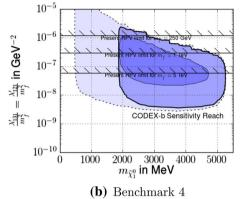
**Fig. 15** Projected sensitivity of CODEX-b for light neutralinos with R-parity violating coupling produced in *D* and *B* meson decays, reproduced from [107] with permission of the authors. The light blue, blue and dark blue regions enclosed by the solid black lines correspond to  $\gtrsim 3, 3 \times 10^3$  and  $3 \times 10^6$  events respectively. The dashed curve rep-
