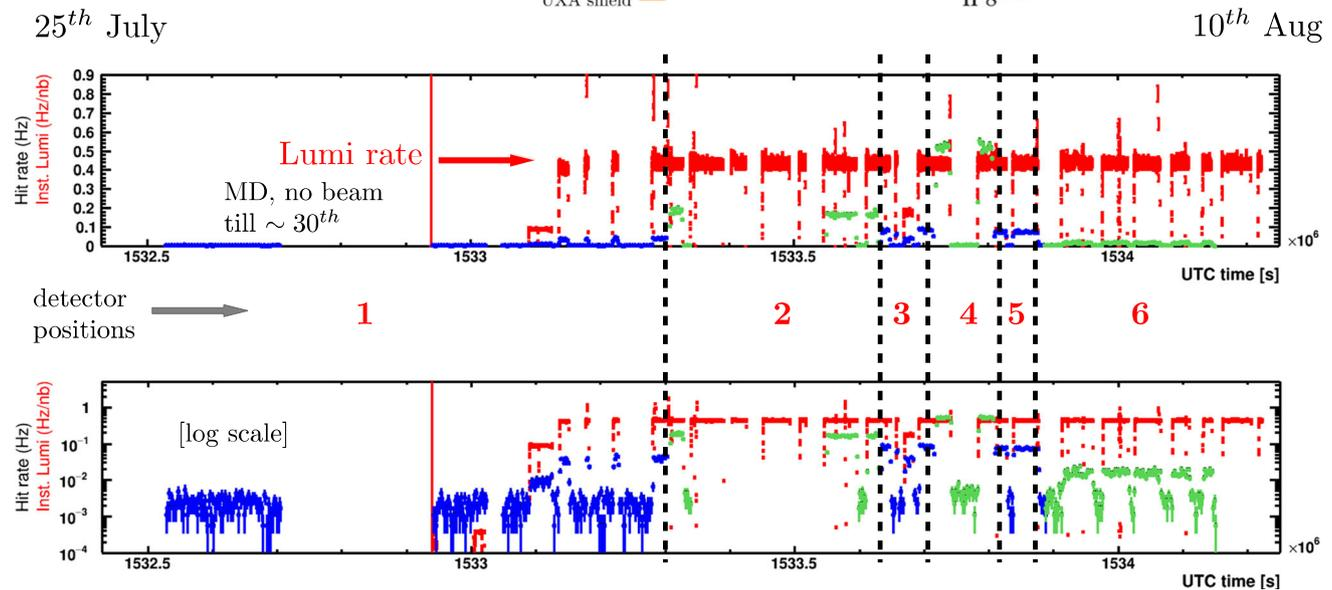
**Fig. 27** Hit rates during the run based on the six P1–P6 positions/configurations on a linear (top) and log (bottom) scale. Red data points denote the luminosity rate of LHCb, blue and green data points denote hit rates. Figure reproduced from Ref. [191]
