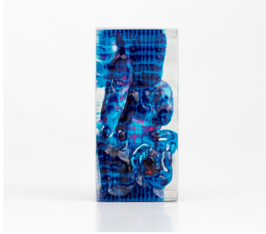
Figure 3-10 voxel model created by Monolith and printed by Stratasys J750
