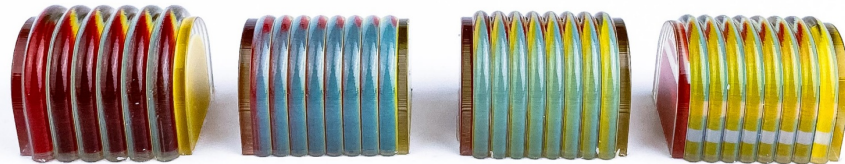
Figure 4-25 lenticular testing with three color-changing content and line pattern on an arched object, with various lens geometry
