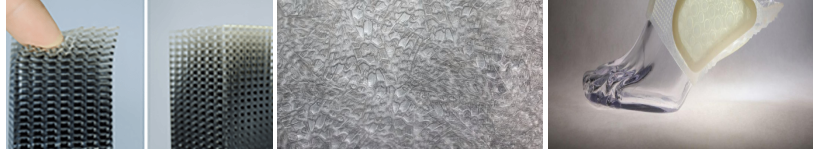
Figure 3-6 left: functionally graded lattice structure with seamless blends of multi-materials (Stratasys, 2017); mid: 3D textile (ibid); right: Voxel Harvest: Metamaterial Programming (Stratasys, 2017)
