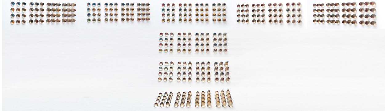
Figure 4-35 viewing printed lenticule blocks in different angles, spherical array testing_2, see Appendix 8 for a high-resolution image
