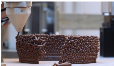
Figure 15. Modulating toolpath speed on 02-03-02
