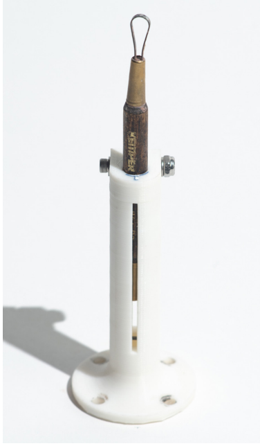
Figure 10. Universal tool holder for carving tools
