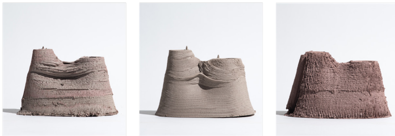
Figure 18. Vaulted geometries realized with different types of nozzle alignment.
