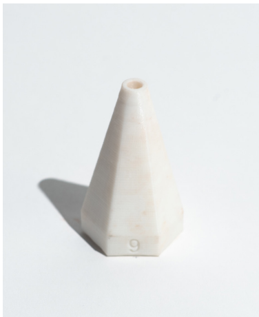
Figure 11. 6 mm nozzle, elongated tip to prevent potential collision
