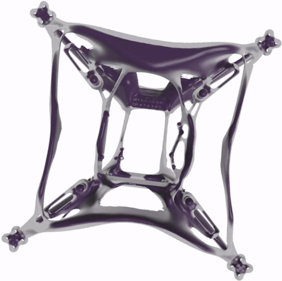
Fig.9 A drone designed by Autodesk using Generative Design methods.
