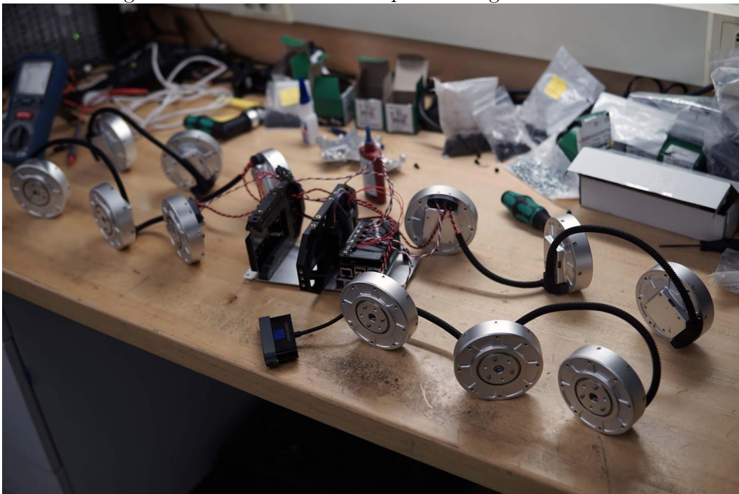
Figure 3-7: Actuator test setup for a single Mini Cheetah
