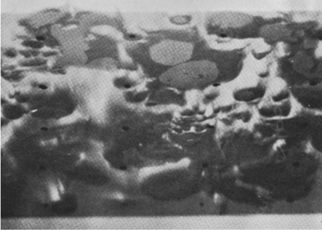
Figure 1.6: Visible Dry Spots on a pool boiling heater at 0.2 bar (fluid: n-heptane). From Van Ouwerkerk [73]
