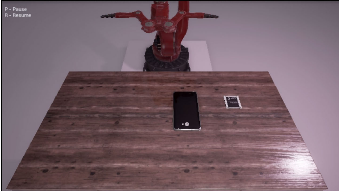
Figure 5-16: Robotic Arm Simulator. The simulator environment consists of a robotic arm placed behind a table, a cellphone and a replacement battery on the table. The simulated perception system sees the environment from the same point of view as in this image.
