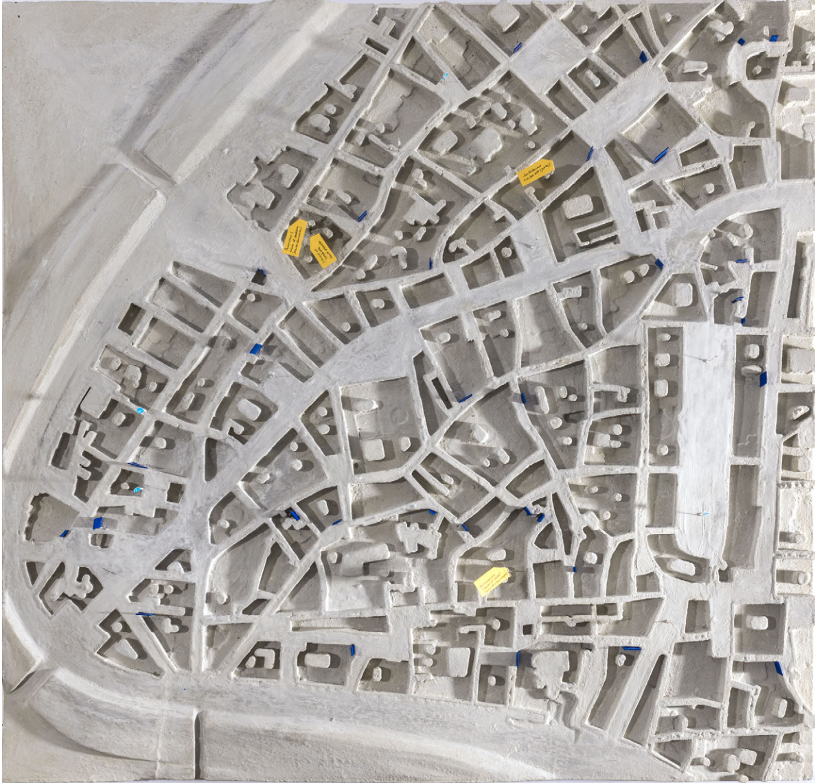
img 46 Site plan noli -style model in concrete. Blue tags mark proposed sites for Third Property Lots and the construction of urban rooms. Yellow tags indicate social services and charities. Light blue pins indicate water fountains. Model photos by Andy Ryan
