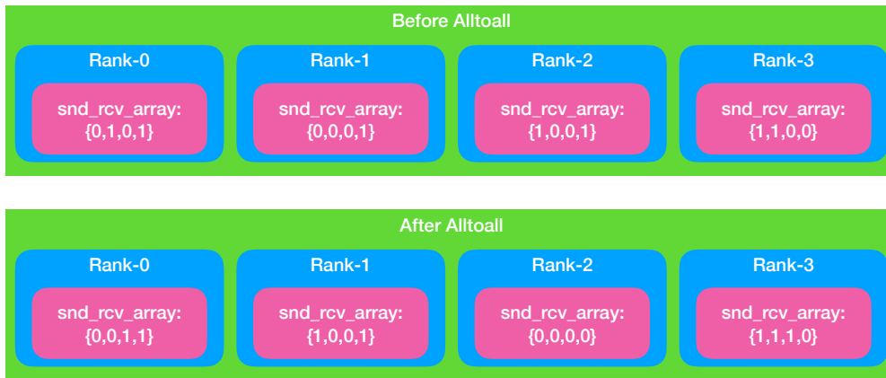
Figure 6.2. Pictorial showing the action of the MPI_Alltoall within the PEX algorithm to notify receivers of who will be sending to them.
