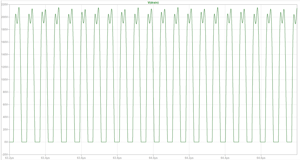
Figure 3-6: Drain to Source Voltage of Phi-2 With Source Model as Load .
