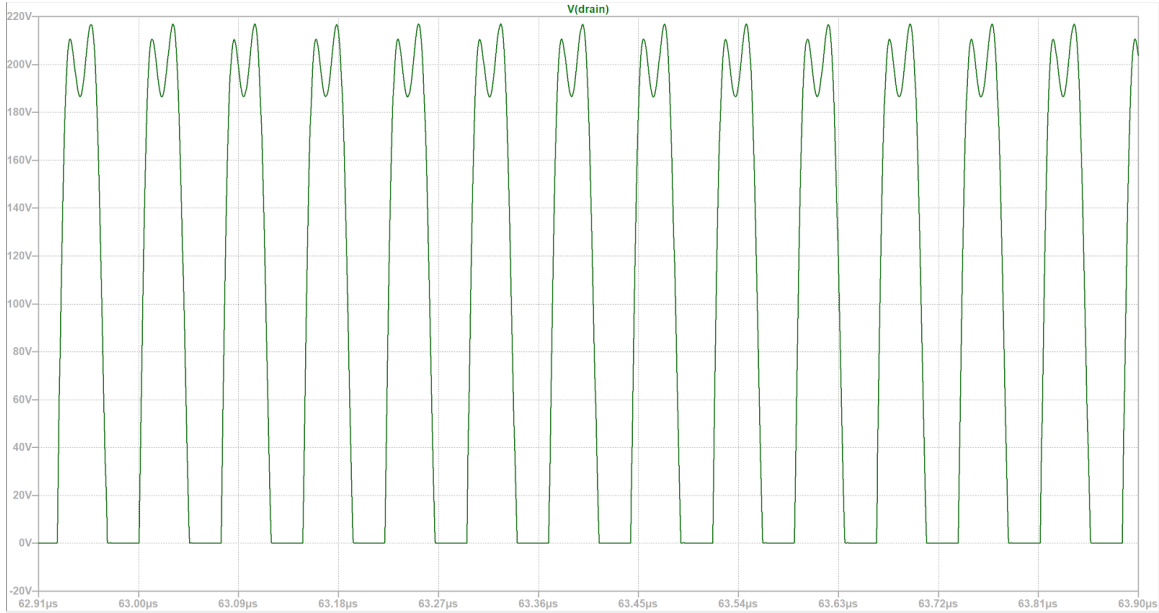
Figure 3-3: Drain to Source Voltage of Phi-2 With Resistive Model as Load.
