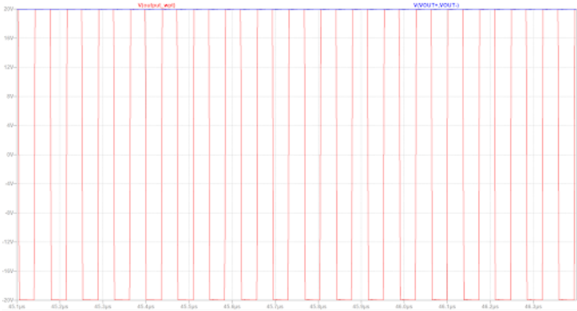
Figure 3-5: Output Voltage of System and Output Voltage of WPT of Phi-2 With Source Model as Load.
