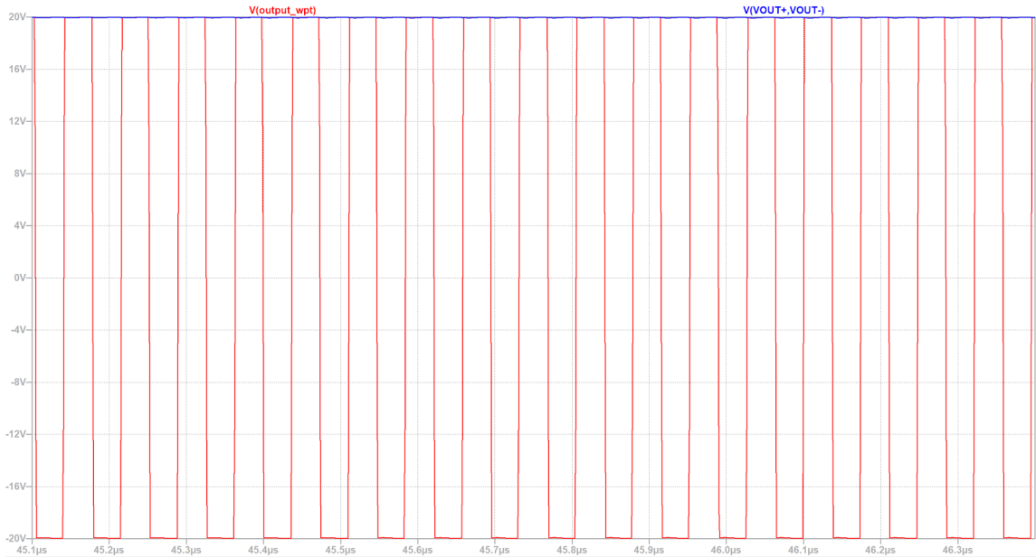
Figure 3-2: Output Voltage of System and Output Voltage of WPT of Phi-2 With Resistive Model as Load.
