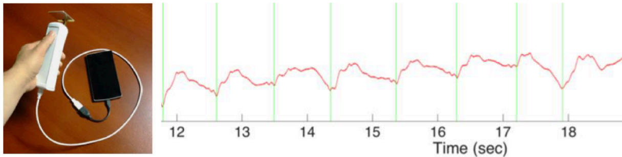
Figure 3.3: Microwave Doppler Sensor (left) and a Sample Collected Signal (right)
