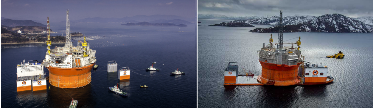
Figure 4-11: BOKA Vanguard transporting the ENI Goliat oil rig to its site in the Barents Sea.
