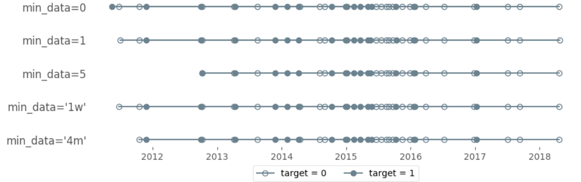
Figure 4-2: The effects of the min_data parameter on the generated target times for a single turbine. If min_data is an integer, it represents the number of entries before starting the search process. min_data can also be a period of time.
