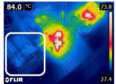
(b) proposed inductor ( \Delta T = \sim 3^\circ\text{C} at P_{out} = 296\text{ W} )
