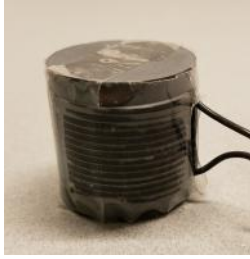
Fig. 11: Prototype inductor of the example design (Section V) having a measured Q of 720. Vertical windows in the outer shell were added to impede the circumferential component of flux and to allow the winding terminations to leave the structure.
