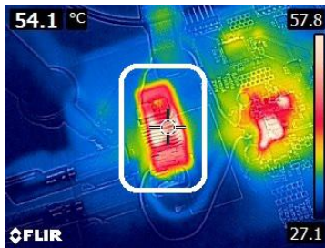
(a) conventional inductor ( \Delta T = \sim 30^\circ\text{C} at P_{out} = 93\text{ W} )
