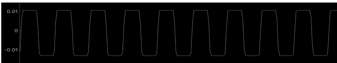
FIGURE 9: ADS1299 INTERNALLY GENERATED TEST SIGNAL UPON REQUIRED CONVERSIONS
