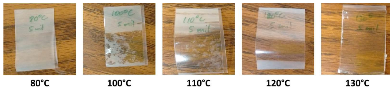
Figure 3-2: Determining minimum viable lamination temperature for EVA/PET film. Temperatures from 80-130°C were tested at a roller force of 50 N and a lamination speed of 2 mm/s. Reproduced with permission from [169].
