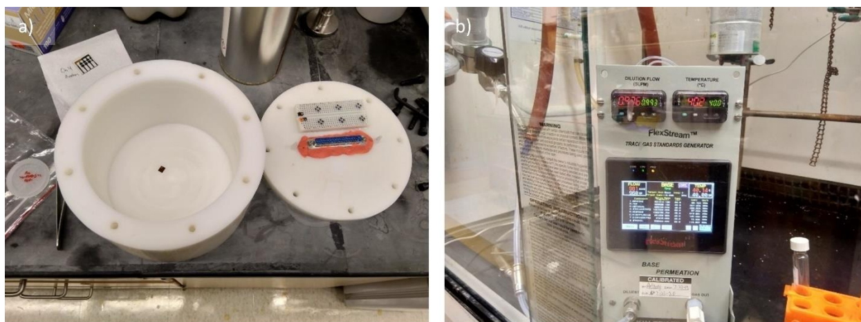
Figure 4-3: Setup for putrescine gas exposure. a) FlexStream™ Base Module from KIN-TEK in a fume hood. b) PTFE chamber for the gas exposure with a chip full of chemical sensors in it.
