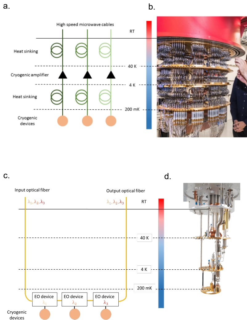
Figure 1-3: Cryogenic readout architectures. (a) Electrical readout. The signal is transported out of the cryostat through the use of high speed electrical cables, requiring amplification and large cable lengths for heat sinking. (b) A dilution cryostat with electrical readout (image from Google). (c) Optical readout. Electro-optical (EO) devices encode the electrical data into an optical carrier transported out of the cryostat through optical fibers. WDM can be exploited to readout multiple data streams with a single optical fiber. (d) A depiction of how optical readout could look like in a dilution cryostat. By reducing the thermal loads and anchoring requirements and exploiting WDM, optical readout can provide a scalable cryogenic readout solution.
