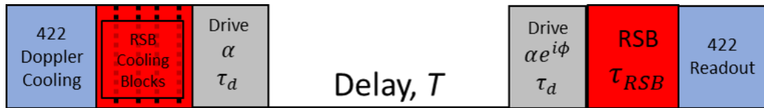
Figure 5-2: Diagram conceptually depicting the sequences of laser and drive field operations applied to the ion, reading from left to right in time. The blocks are not to scale in time.
