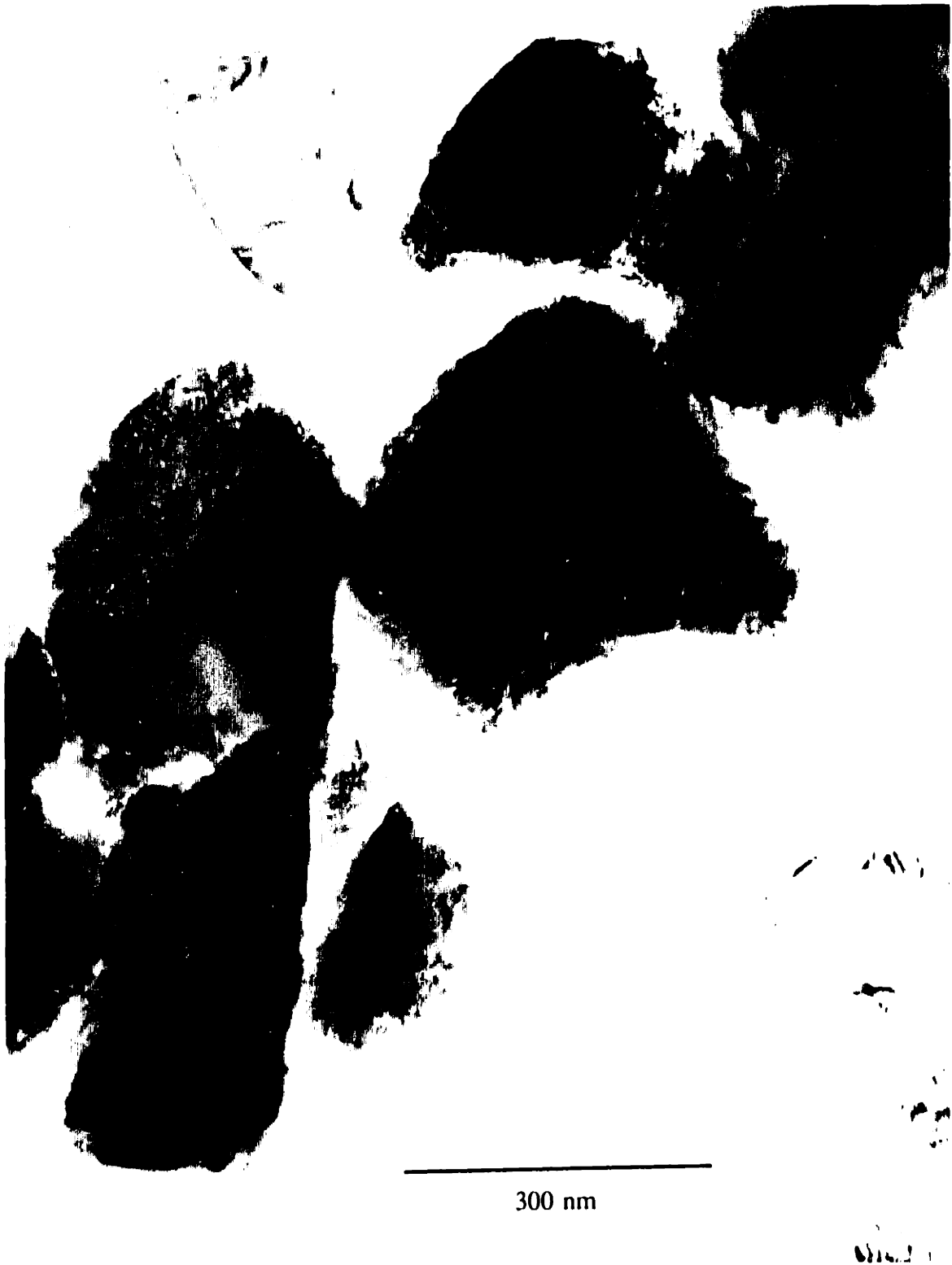
Figure 5.9. TEM micrograph of alumina particles from R1.
