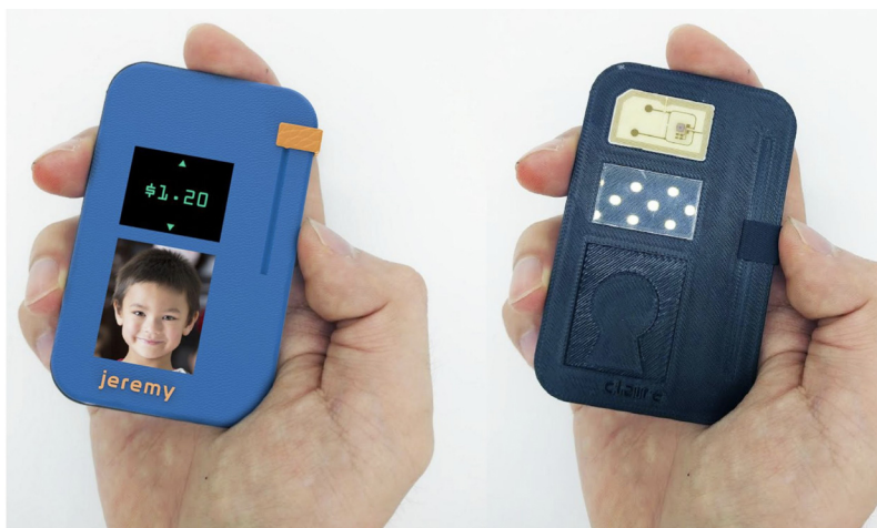
Fig. 13 A single design concept was realized as a physical prototype (right)—to demonstrate its interactivity—and also as a rendered image (left) to illustrate its visual elements; each eliciting different design information
