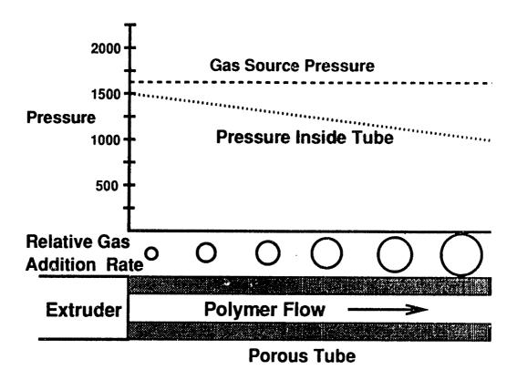
Figure 3-1: Pressure Profile Along Length of Porous Tube, Showing Relative Gas Addition Rates
