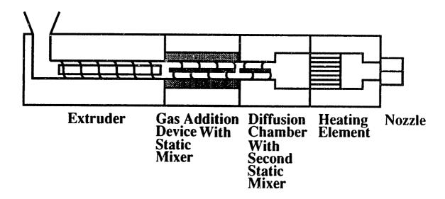
Figure 4-1: Schematic of MFP Manufacturing Process
