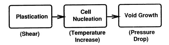
Figure 2-1: Schematic of MFP Process
