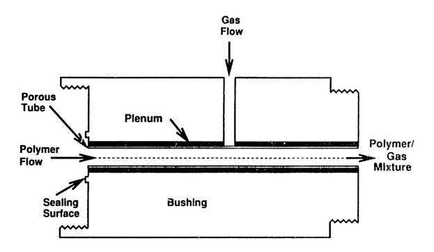
Figure 4-3: Schematic of Gas Addition Device
