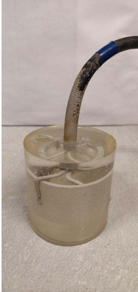
**Figure 2-19:** PU Potted 25kHz piezoceramic transducer with soldered PU jacket 4 conductor cable
