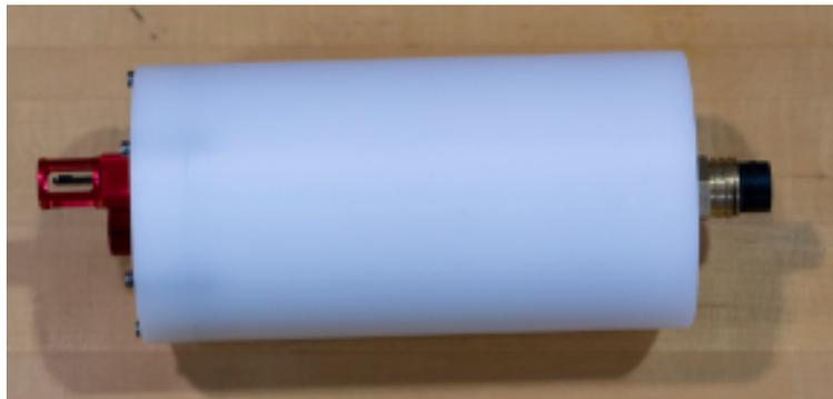
**Figure 2-54:** OpenModem Pressure Housing
