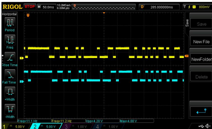
Figure 4-10: The yellow trace is the transmission digital signal at 100 bits per second, and the blue trace is the decoded DBPSK output
