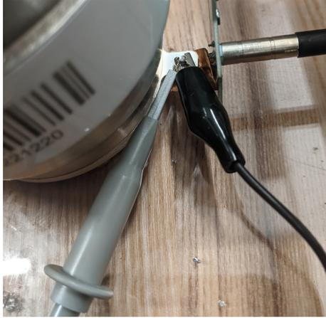
Figure 5-7: “Ground to Ground” Probe. The voltage measured on the oscilloscope is indicative of common mode ground currents.
