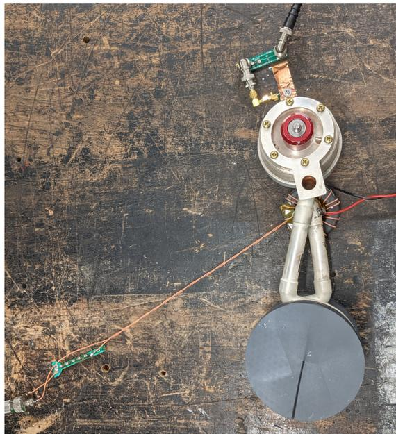
Figure 5-6: Birds' Eye View of Transformer Coupled Resonant Tank Test Fixture. The green PCB in the bottom left of the photo houses  $C_{\text{leak}}$ . By manually tuning this capacitance, the impact of the transformer's primary-referred leakage inductance can be nulled.
