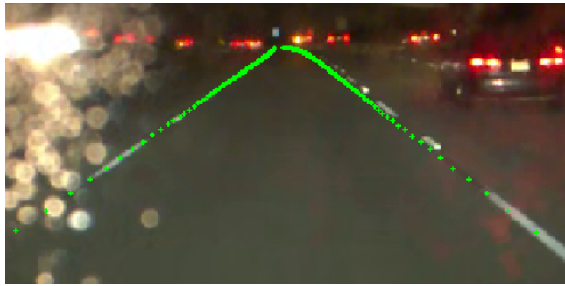
(a) The dashcam image with the proposed lane lines (green) superimposed on the image.
