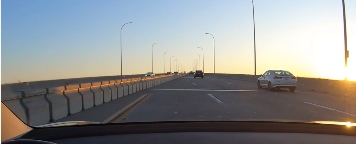
Figure 3-1: An image taken from dashcam footage in which a car using Tesla’s autopilot almost ran into a concrete barrier. The malfunction was presumably caused by the perception system mistaking the reflection along the barrier for a lane line.
