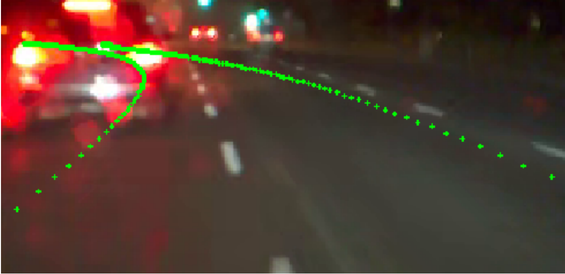
Figure 2-3: An example of a lane-detection failure detected by the monitor. The green lines represent the proposed lane lines.
